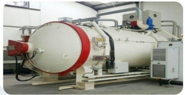
❖ VACUUM HEAT TREATMENT -01 Nos
